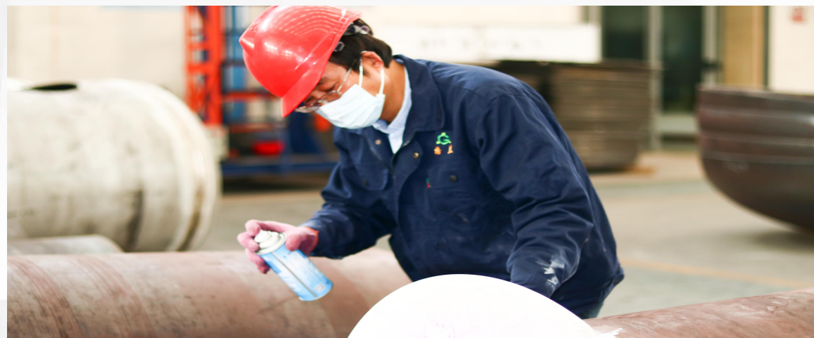
渗透检测 Penetrant testing
