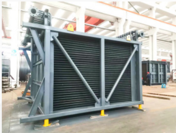
Tubular air preheater
