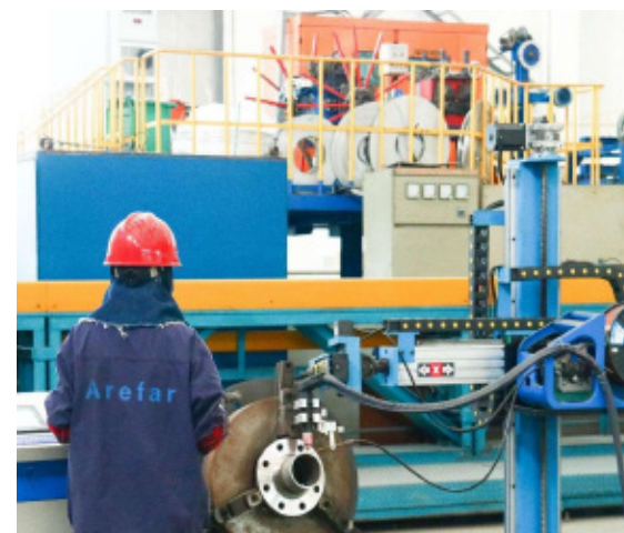
Automatic welding machine for connecting pipe flange
