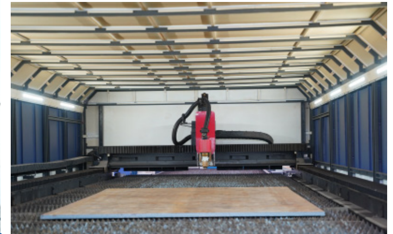
40000W Laser Cutting Machine (Double Material Table)
